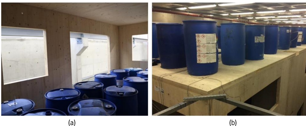
Figure 4.3 – Additional masses used in the tests. (a) 1 st floor; (b) 2 nd floor.
