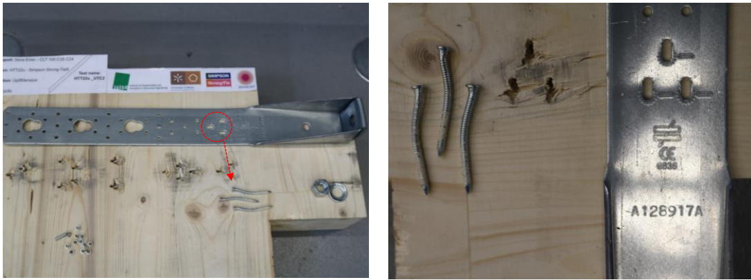
Figure 3.27 – Failure of the hold-downs HTT22E under tension loads.
