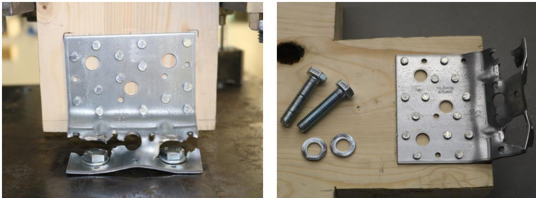
Figure 3.20 – Failure of the angle brackets under tension loads fixed to a steel plate support.
