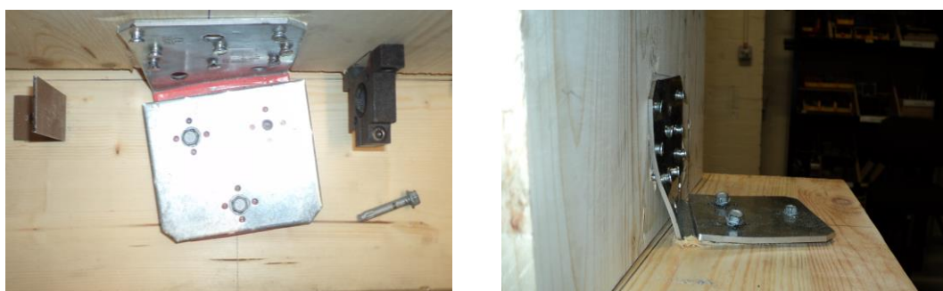
Figure 3.31 – Failure of the angle brackets AB+plate under lateral loads.
