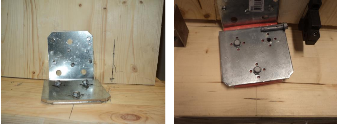
Figure 3.32 – Failure of the angle brackets ABAl under lateral loads.
