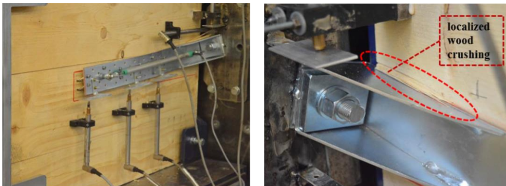
Figure 2.29 – Failure mechanisms of the hold-downs WHT 540 analyzed under axial-shear interaction [42].
