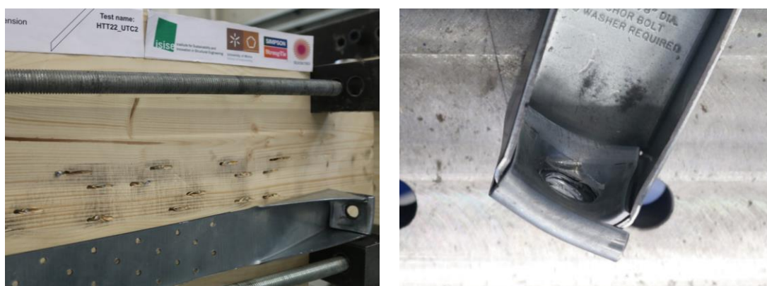
Figure 3.26 – Failure of the hold-downs HTT22 under tension loads.
