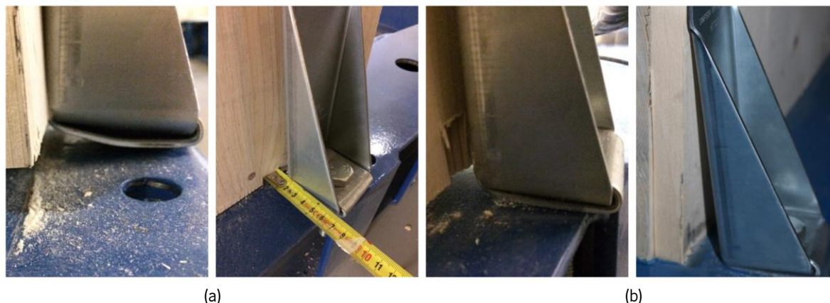
Figure 4.17 – Damages observed in the HTT22 connectors: (a) Monotonic transverse direction; (b) Cyclic transverse direction.
