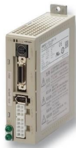
Figura 4.6 - Driver OMRON R7D-BP02HH .
