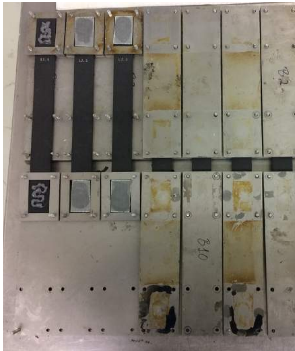
Figure 13: Tabs attachment on tensile specimens.
