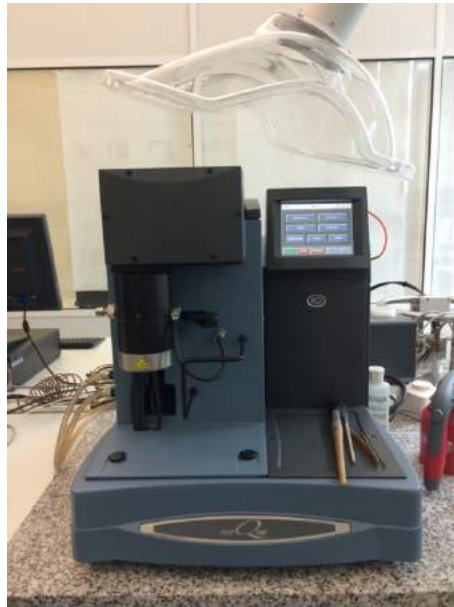
Figure 20: TGA Q500 gravimetric balance.
