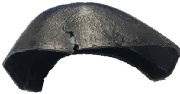
Figure 5.31 – A nose cap made from 19% FVF pellets after the compression test
