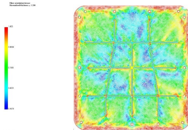
Figure 7.6 - Fibre orientation tensor results for a compression moulding simulation. A red colour indicates a highly oriented fibre orientation while blue colour indicates a 2D random orientation.
