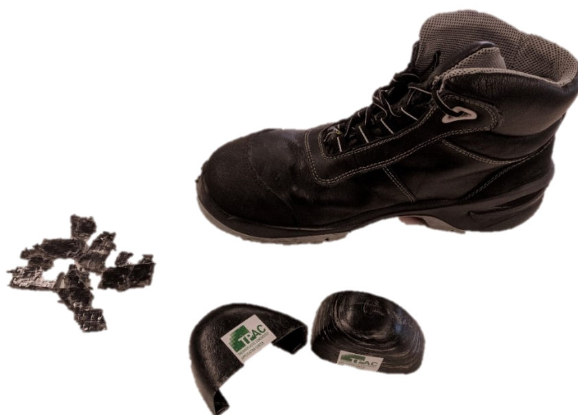
Figure 5.17 - The shredded flakes (left), a safety shoe (top) and the developed nose caps (bottom)
