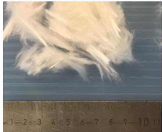
Figure 5.29 - The glass fibres of a nose cap made of recycled flakes after the resin is burned out show long fibres in random orientation
