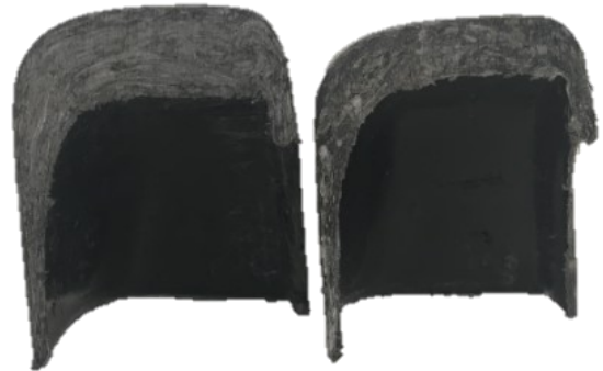
Figure 5.25 - Cross section of nose caps with a thickened front (left) and normal (right) FVF 35%
