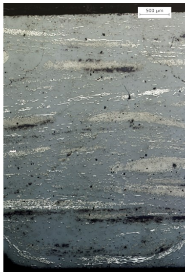
(b) Mixed cut semipreg at 20% FVF
