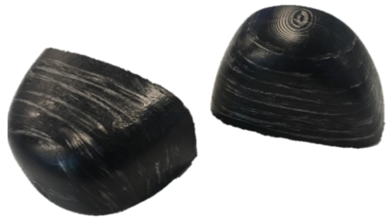
Figure 5.25 - Cross section of nose caps with a thickened front (left) and normal (right) FVF 35%
