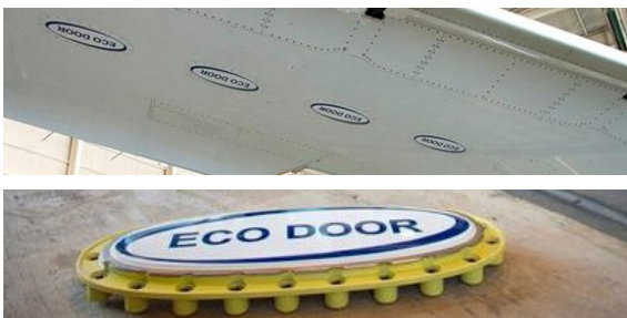
(c) Wing-access panels (bottom image) mounted on the Boeing ecoDemonstrator 787 flight-test airplane wing (top image) reclaimed carbon fibre material. Photo by John D. Parker and Image courtesy: The Boeing Co. [111].
