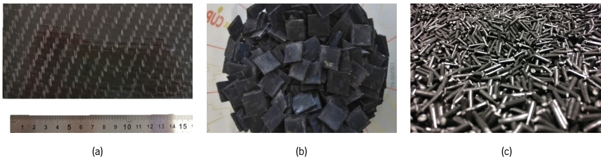
Figure 4.4 - G/PP consolidated laminated (a), cut consolidated flakes (b) and UD LFT pellets (c)
