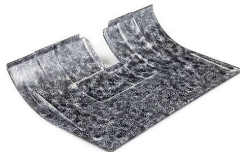
(b) Access panel with integrated design features like ribs, joggle and thickness transitions. The part is made out of C/PPS semipreg flakes by DCM. Image courtesy TPRC / Rasheed [5].
