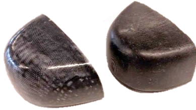
Figure 6.16 - Two Safety shoe nose caps: left cap made of virgin glass/epoxy, right cap made of recycled G/PP
