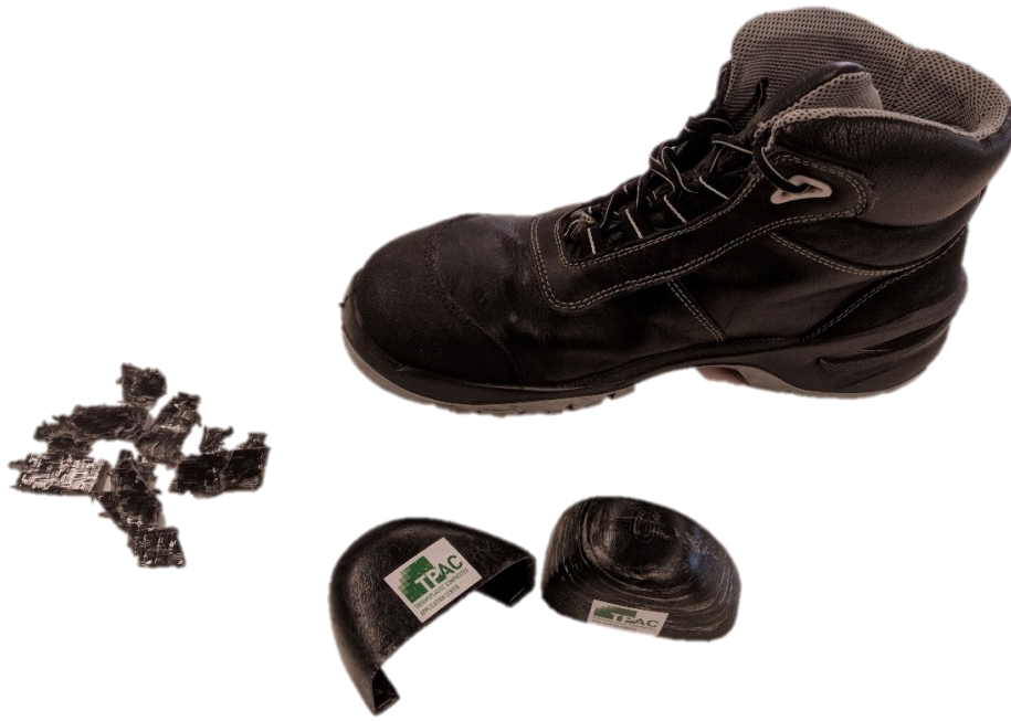
Figure 6.15 – Safety shoe application with shredded material (left), a safety shoe (top) and the G/PP nose caps (bottom)
