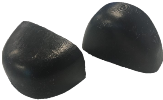
Figure 5.24 - Produced nose caps of recycled material with 19% FVF
