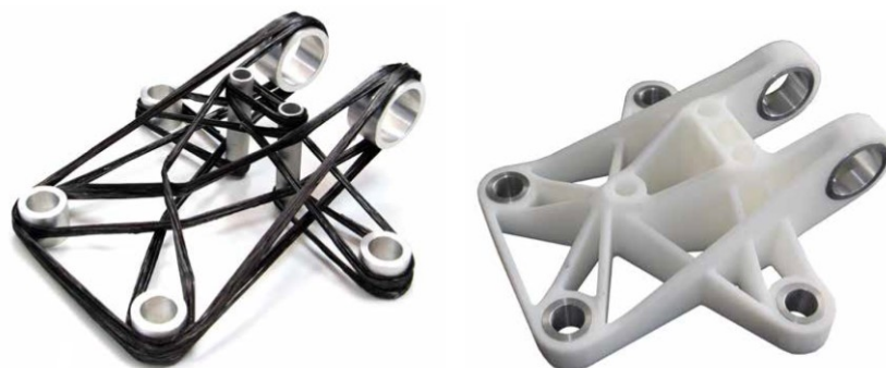
Figure 5.41 - A UD tape insert wound around bushings for the fasteners (left) and an over moulded bracket (right). Image courtesy Fraunhofer ICT [25]
