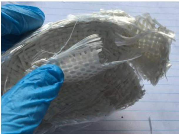
Figure 5.28 - The glass fibres of the benchmark nose cap after the resin is burned out show a structure of multiple patches
