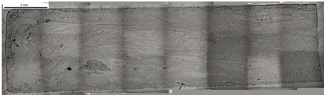
Figure 4.25 - Cross section showing the edge of a compression moulded mixed pellet plate with 35%v fibre content.
