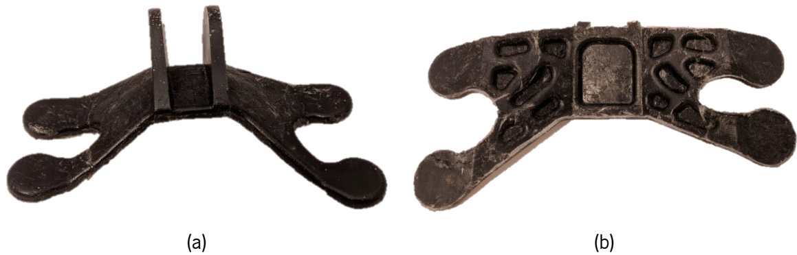
Figure 5.40 - The top (a) and bottom (b) view of a produced bracket from G/PP material
