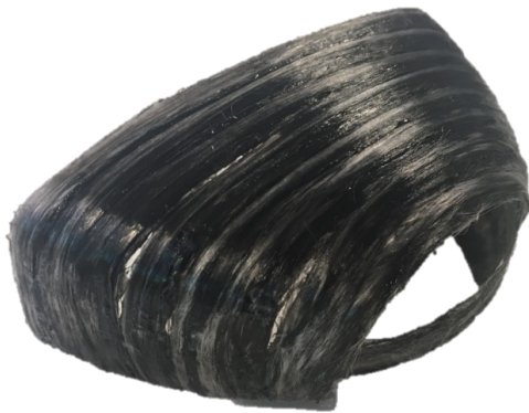
Figure 5.24 - Produced nose caps of recycled material with 19% FVF
