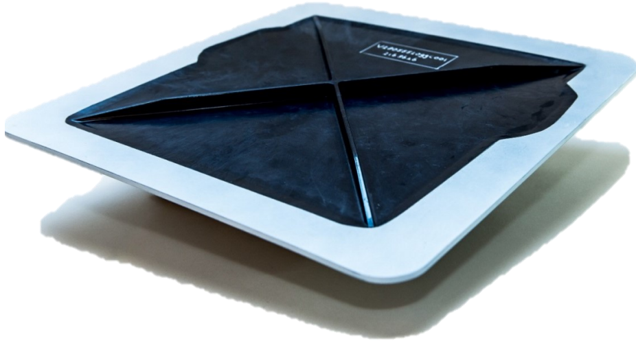
Figure 5.14 - Designed and manufactured access panel for the rotorcraft. The landing area is coated with a light blue primer.
