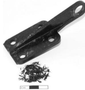
b) A rotorcraft door hinge made of C/PEEK flakes obtained by Electrodynamic fragmentation. Source Roux et al. [6]
