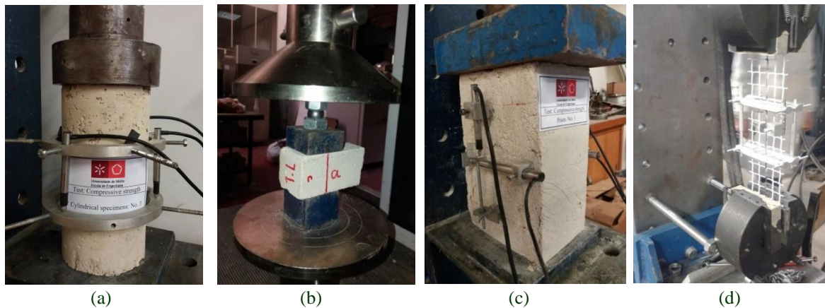
Figure 3. Characterization of the masonry and strengthening materials: (a) compression test on a cylindrical specimen casted from the adobe mixture; (b) compression tests on strengthening mortar specimen; (c) adobe masonry prism tested under compression; (d) fiber-glass mesh tested under direct tension.
