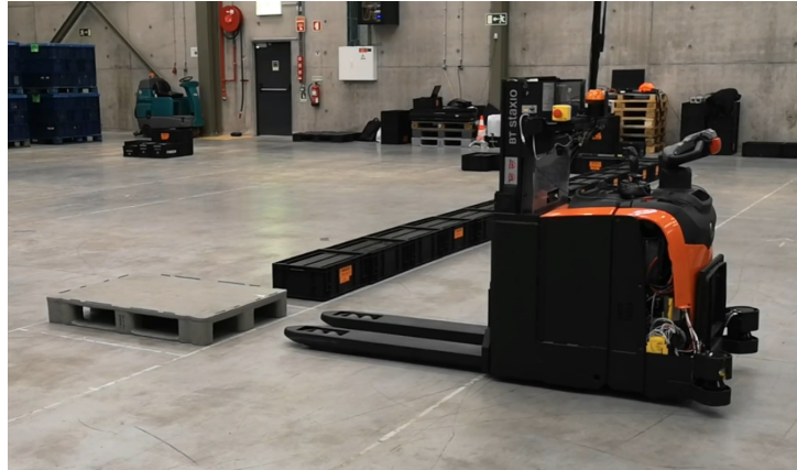
Figure 1: A stacker getting ready to pick a pallet
