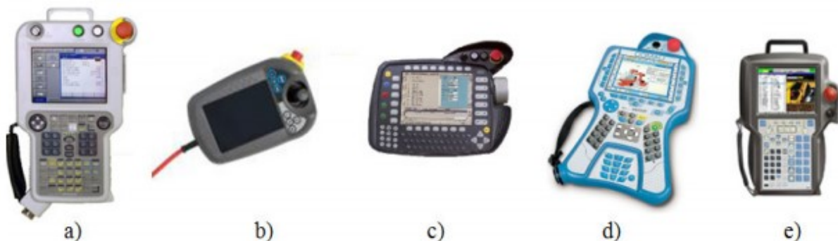
Figure 2.2: Robot teach pendants: a) the MOTOMAN NX100 teach pendant; b) the ABB IRC5 teach pendant that incorporates a joystick; c) teach pendant from KUKA Robotics incorporating a 6D mouse; d) wireless teach pendant from COMAU Robotics; e) FANUC robot tech pendant[Neto et al. (2010)]
