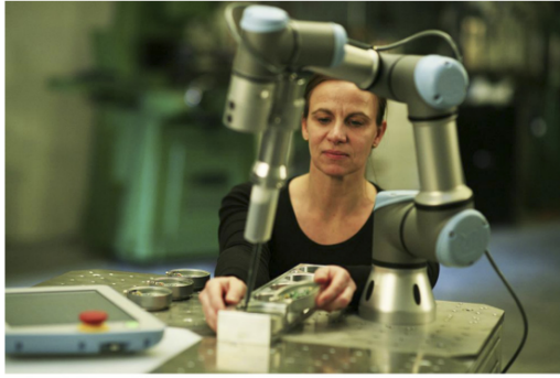
Figure 1.2: On the left, cobot UR3 in a collaborative gluing application [Bloss (2016)]; On the right conventional industrial robot in a non-collaborative workspace [Tsarouchi et al. (2016)].
