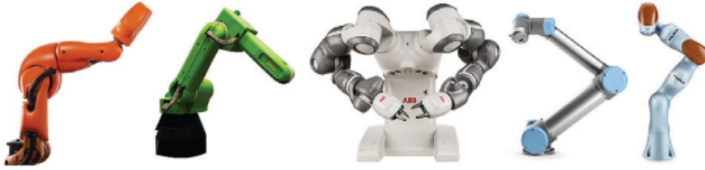
Figure 1.3: Collaborative robots – MRK-Systeme KR SI, Fanuc CR-35iA, ABB YuMi, UR5, KUKA LBR iiwa [Vysocky and Novak (2016)]
