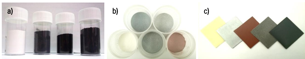
Figure 2.2 | Visual aspect of the materials prepared: a) M-samples containing CNT; b) M-samples containing metal particles; c) P-samples from respective M-samples containing metal particles, from left to right: P-PA6, P-Al10, P-Cu10, P-Mg10, P-Fe10.
