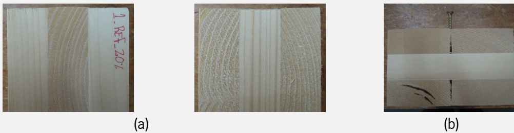
Figure (I) 3:23. Damages caused by high MC levels. (a) deformations on CLT shape caused by timber swelling depending on grain direction; (b) closing of GAP4 after conditioning period.
