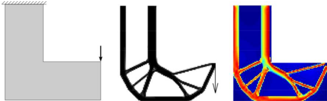
Figure 4.1 - Structural optimization of an L-shaped beam subject to global stress constraints, Erik Holmberg, University of Linköping .
