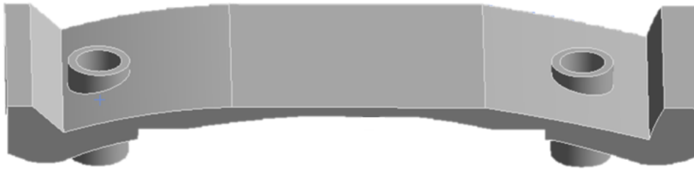
Figure 5.19 – Geometry obtained at the redesign process and inspired by the stl file obtained through the Topology Optimization operation performed previously.
