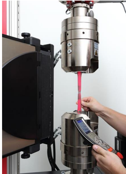
Figure 4.16 - Uniaxial tensile testing equipment. Although this photo is not exactly the model present in the University of Minho's laboratories, it is quite similar.
