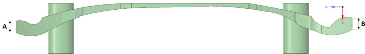
Figure 5.25 - Identification of the two main parameters to be optimized by genetic algorithms. The letter "A" represents the thickness of the left attachment zone and the letter "B" the thickness of the right attachment zone.
