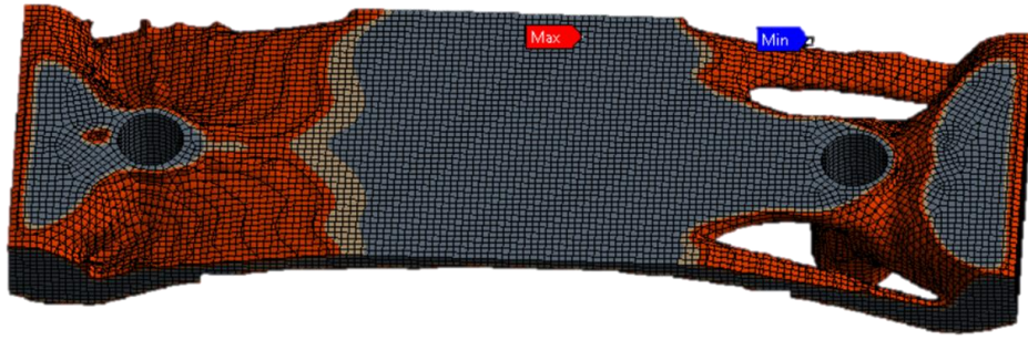
Figure 5.17 - Geometry obtained after the first cycle of Topology Optimization and based on Initial Geometry 1.2. The geometry represented has a mass of 18.5 kg.
