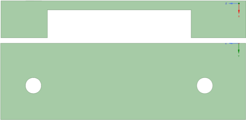
Figure 5.4 - Second version of the initial geometry that will undergo topology optimization processes. In this case, some design limitations were considered, for example, the lower surface of the component was required to be available for fixing other components. This geometry will be referred to as initial geometry 1.2.
