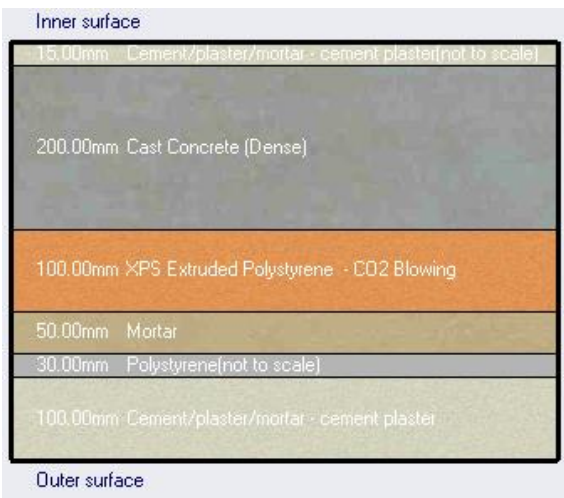
Figure 140. Building materials used in the new proposed units, roof materials
