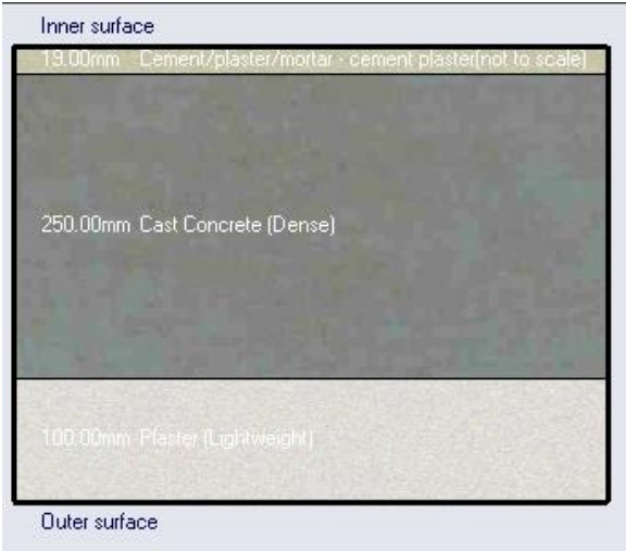
Figure 125. Materials used in the first design simulation, the roof of the building
