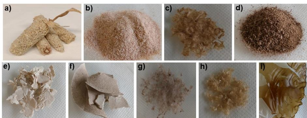
Figure 4-2. Photographs of (a) corncob, (b) ground corncob, (c) ionic liquid treated corncob, (d) LHW treated corncob, (e) NaOH treated corncob, (f) LHW-NaOH treated corncob, (g) LHW-NaOH-IL treated corncob, (h) NaOH-IL treated corncob and (i) LHW-IL treated corncob.
