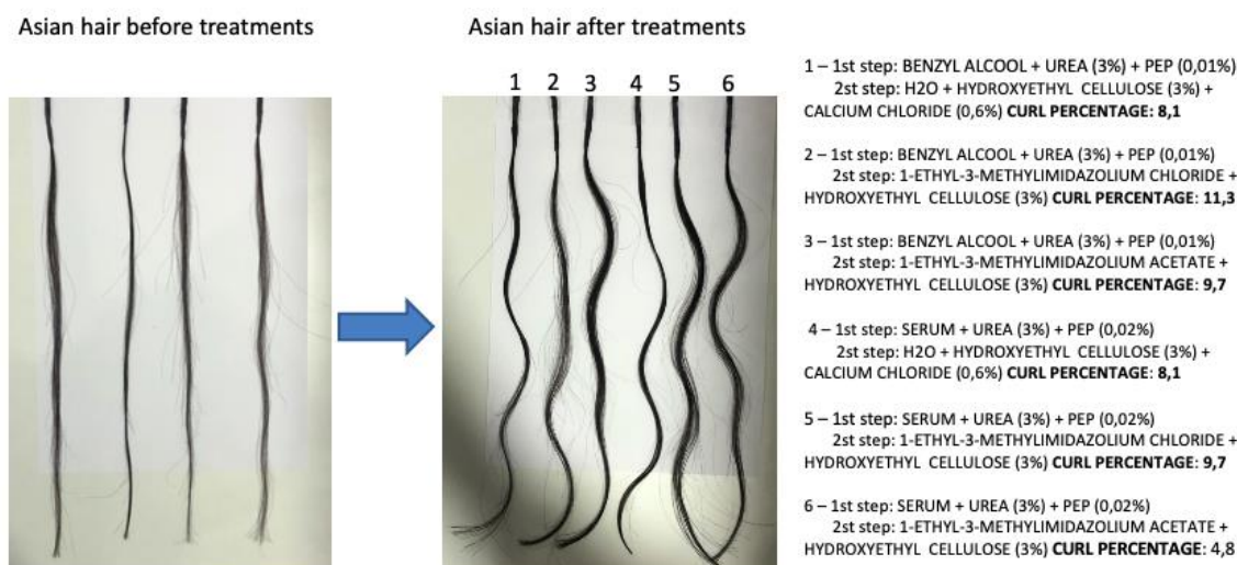
Figure 23: Visual curl formation on Asian hair using the methodology referenced as number 3 (after wash), including a first step pre-treatment with urea followed a second step with treatment containing cellulose in ionic liquid and in water.
