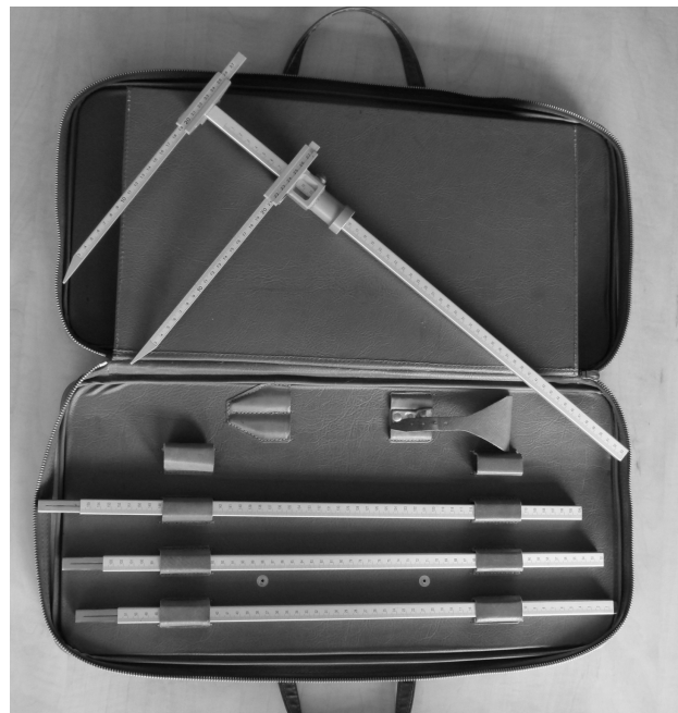
Figure 2.2. Martin type anthropometer
