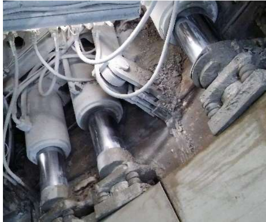
Fig.26-Grippers pressionados contra as aduelas [58]
