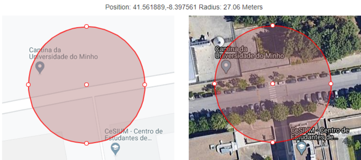
Figure 3.3: Range of the second-generation ESP8266 ESP-12E NodeMCU Amica board within a point-of-interest for VRUs: a pedestrian crossing.
