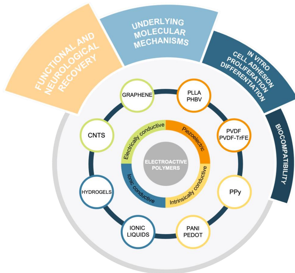
Figure 1. Schematic overview. Electroactive polymers can be subdivided according to their conduction mechanism into electronically conductive polymer composites, piezoelectric polymers, ionic conductive polymers and intrinsically conductive polymers. Overall, studies focusing on electroactive-based approaches for neural regeneration are devoted to the evaluation of the biocompatibility of the materials, in vitro and in vivo performance and underlying molecular mechanisms for neuroregeneration 13,21,47,58 .
