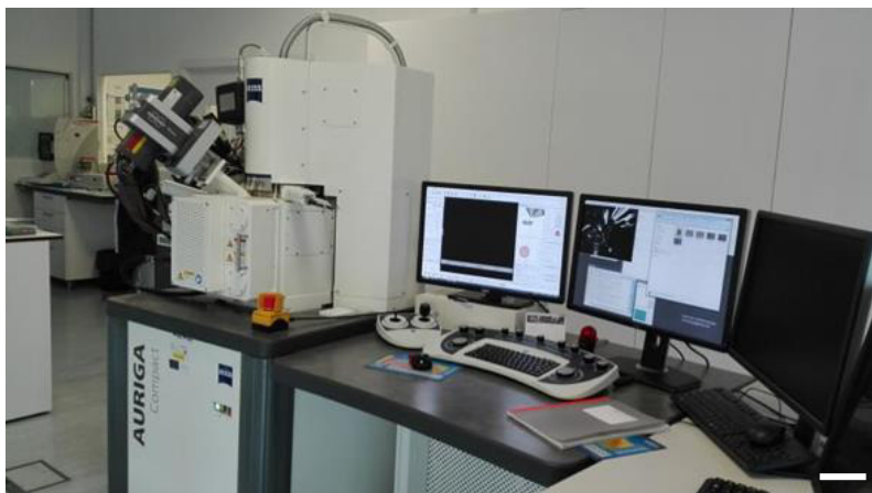
Figure IV-13 - The AURIGA compact is a FIB-SEM instrument combining the powerful imaging and analytical performance of field emission scanning electron microscope (FE-SEM) with the superior processing ability of Focused Ion Beam (FIB). Scale bar: 10 cm.
