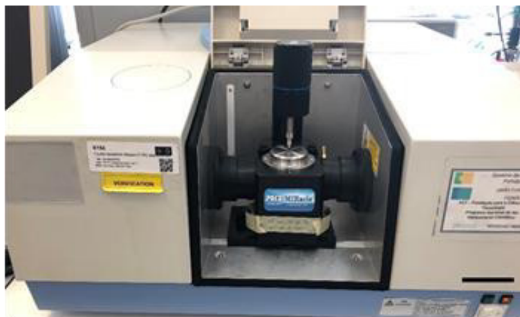
Figure IV-10 - The Fourier transform infrared (FTIR) spectrometer is used as a standard chemical characterization technique. The samples can be analyzed as films, KBr discs, powder or liquids. The available methodologies comprise transmittance, specular reflectance, diffuse reflectance and attenuated total reflectance (ATR). Scale bar: 10 cm.
