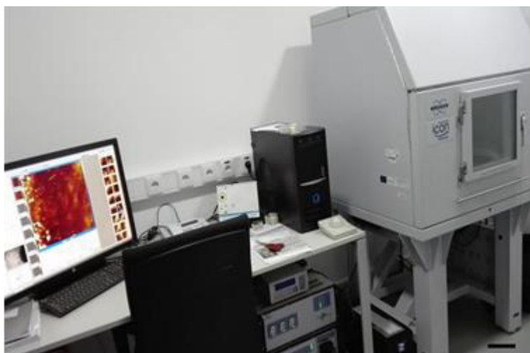
Figure IV-12 - The AFM allows acquiring images of flat surfaces that can encode the surface topography, mechanical response, among other properties. Scale bar: 10 cm.
