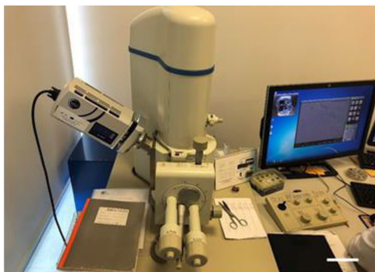
Figure IV-11 - The SEM with EDS analyzer. The SEM (JSM-6010 LV, JEOL, Japan) instrument is equipped with an energy dispersive spectroscope (EDS). Scale bar: 10 cm.
