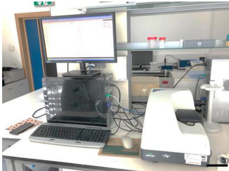
Figure IV-14 - Zetasizer Nano ZS, Malvern Instruments. Scale bar: 10cm.
