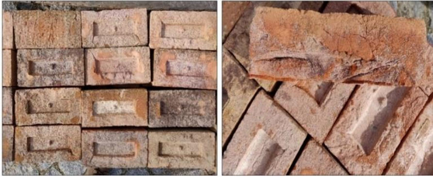
Figure 20: Solid molded clay brick with frogs chosen for the project, supplied by Wienerberger
