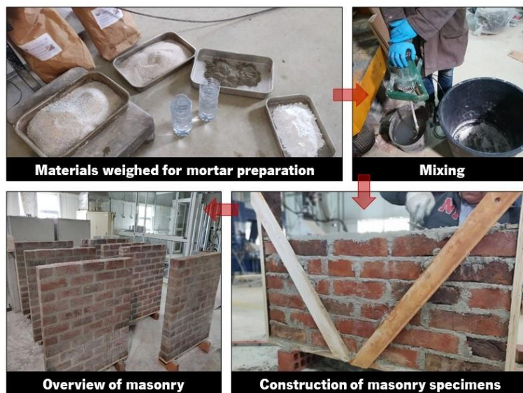
Figure 26: Illustration of process used to construct masonry
