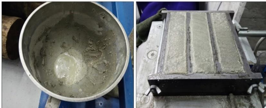
Figure 25: Water expelled (a) during compaction from a trial of the reference cement mix (b)
