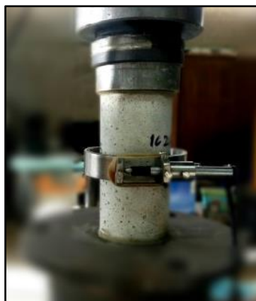
Figure 56: Measurement of Poisson's ratio - Set up of the specimen with the horizontal layout of LVDT
