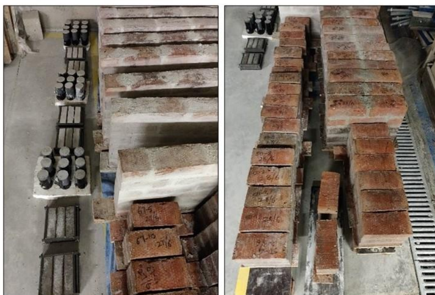
Figure 28: Left – Mortar specimens constructed for in situ characterization with masonry | Right – Overview of masonry specimens cast for mechanical characterization
