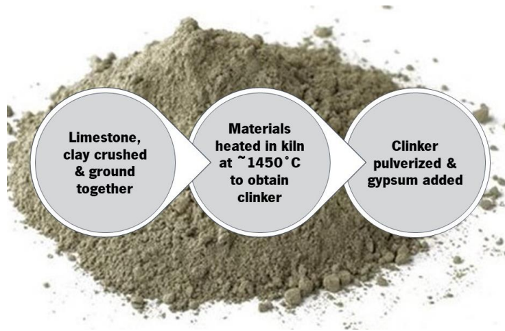
Figure 3: Depiction of the process of cement production
