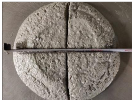
Figure 23: Target consistency aimed for 175 \pm 10 mm, for all mortars
