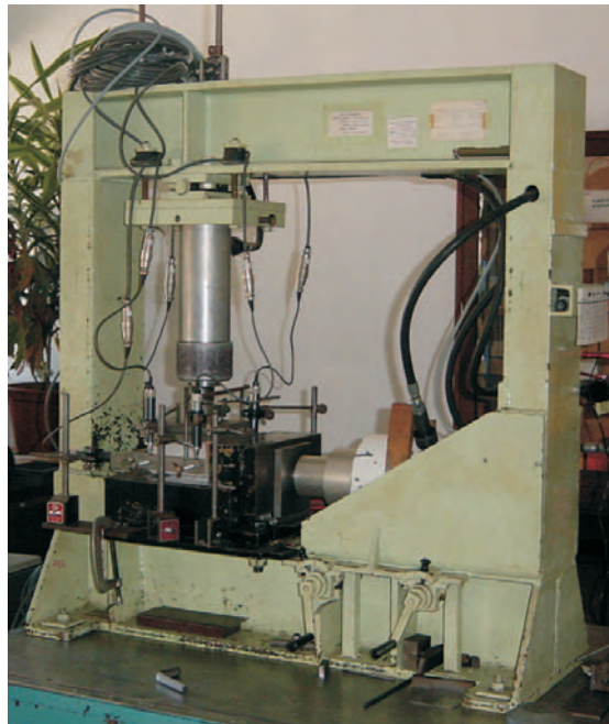
Figure 2.5: Equipment for sliding test in discontinuities of LNEC
