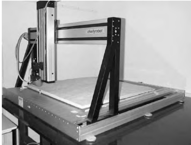
Figure 2.6: 3D laser scanner for measuring the topography of joint surface (Fardin et al. , 2001).
