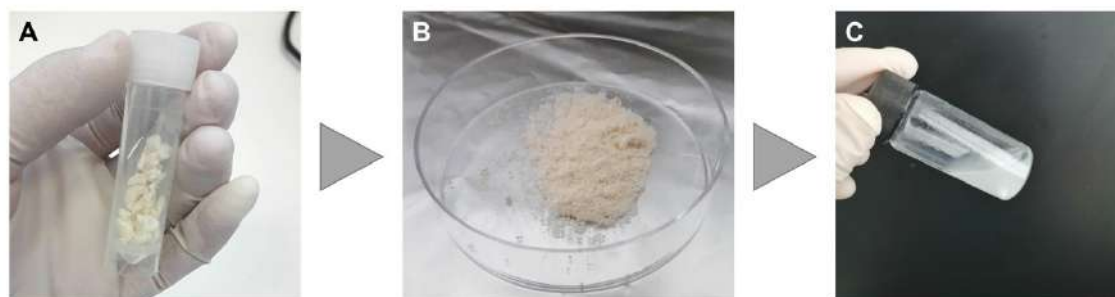
Figure II-4 - Schematic representation of the processing steps after the decellularization process. The matrix is lyophilized (A) and ground into a fine powder (B) which is then solubilized in a pepsin-containing acidic solution, acquiring a gel-like consistency (C).
