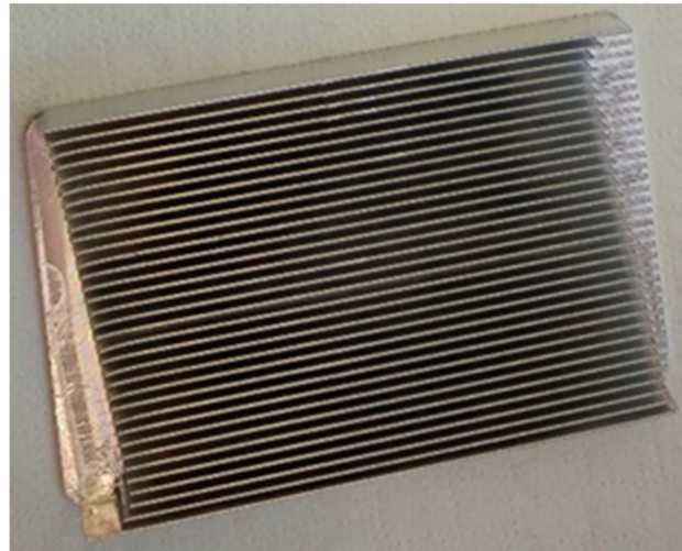
Figure 5. Example of affordable extruded finned heat sink SK624 from Fischer Elektronik [28], which has been adapted by the authors for liquid cooling by adding a cover and hoses and by machining inlet and outlet collectors.
