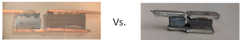
Figure 3. Copper and aluminium connectors implemented in silicide-tetrahedrite TE pairs.
