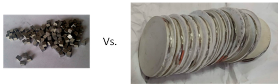
Figure 2. Example of small vs. large TE element, with 24 mm diameter BiTe elements.
