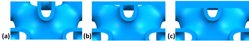
Figure 30 - Shell thickness of Neovius samples: a) without shell (NS1), b) 1 mm (NR) and c) 2 mm of shell thickness (NS2).
