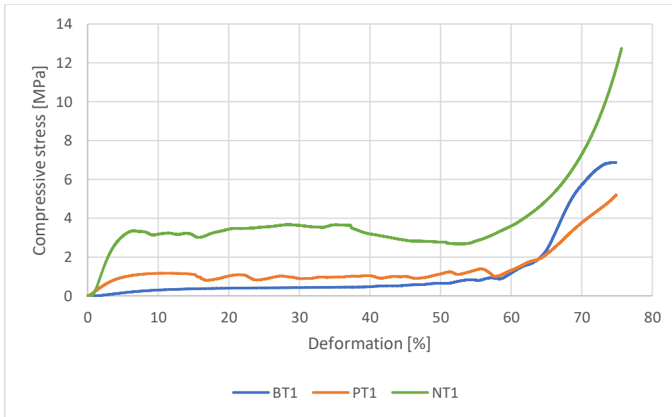
Figure 34 - Compressive stress-strain curves of lower surface thickness (T1).
