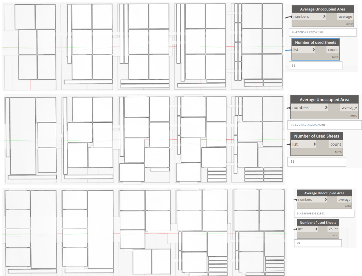
Figure 4.23 – Panelization optimized layout with Area Packing Strategy (top -RefineryToolkits), LongSide Packing Strategy (middle -RefineryToolkits), ShortSide Packing Strategy (bottom - RefineryToolkits)
