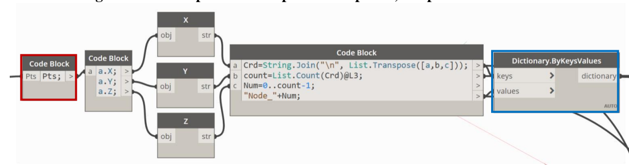
Figure 5.27 – Graph definition part: Node Dictionary creation. Input node in red frame is the output from Figure 5.26
