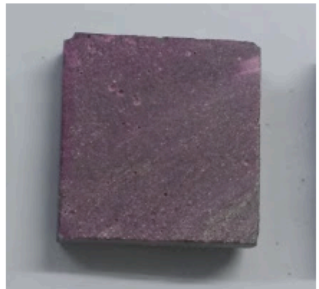
Fig. 9. Freshly split surface of a UHPC sample with ECat incorporation sprayed with the phenolphthalein solution after spent 12 months in an accelerated carbonation chamber (pink surface indicates no-carbonation occurrence). (For interpretation of the references to colour in this figure legend, the reader is referred to the web version of this article.)
