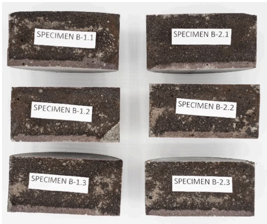
Fig. 8. Split surfaces of cylinder samples after the rapid chloride permeability test at 28 days; chlorides ingress from the side of the bottom surface (penetration depth of chloride ions in the lighter part).
