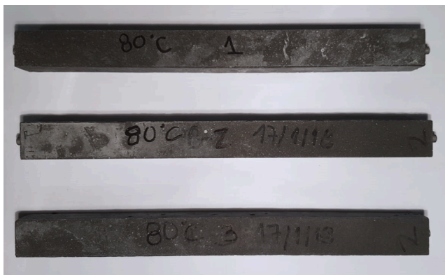
Fig. 11. UHPC samples (Set 1) after long term ASR test.
