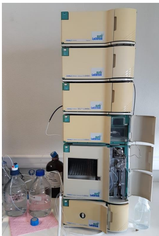
Figure 3. Method of separation (HPLC) used in this work. The system is composed by a UV detector, a column oven, an auto sampler, and a pump.
