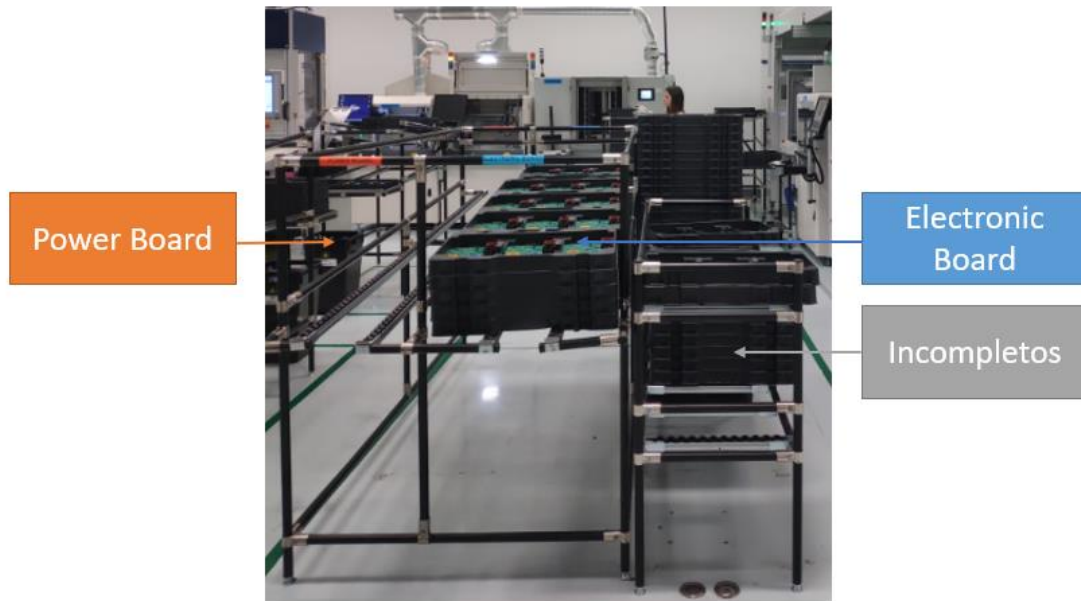
Figura 111 - Rampa de coating FIFO
