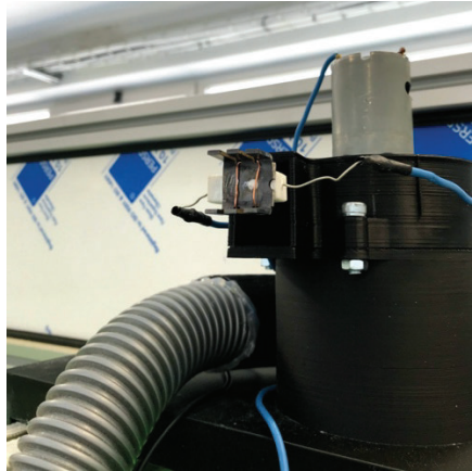
Figure 4.35. Resistor used in the suction system circuit.
