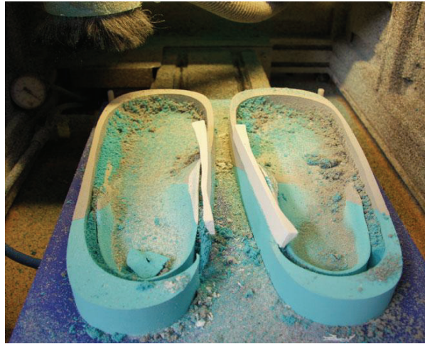
Figure 3.36. Insoles machined by 'London Orthotics' (London Orthotic Consultancy, 2020).
