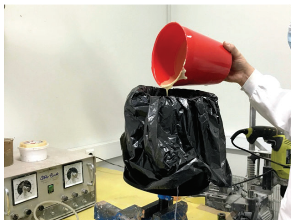
Figure 3.31. Leakage of the mixture into the container resulting in the mould block.
