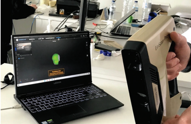
Figure 3.22. Scanning baby's head with 'EinScan-Pro+'.
