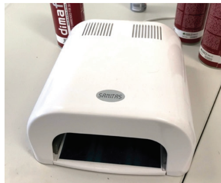
Figure 4.25. UV nail dryer used for the resin part hardening.
