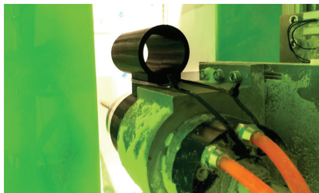
Figure 4.38. Tube holder assembled to the spindle with a clamp support.
