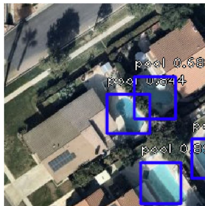
Figure 2.33: Filtered bounding boxes according to the threshold value chosen by the user.
