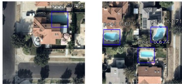
Figure 5.8: Model's predictions of two testing images of the dataset using ResNet152 as backbone architecture.
