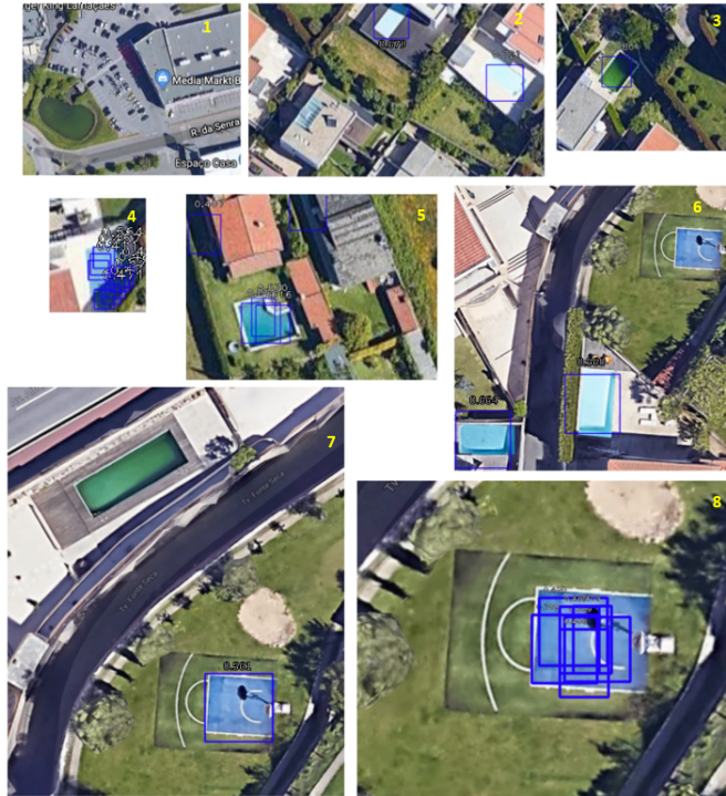
Figure 5.11: Eight test images taken from google maps with different sizes and resolutions. The detected objects are enclosed by blue boxes. The images are numbered on the top right corner.
