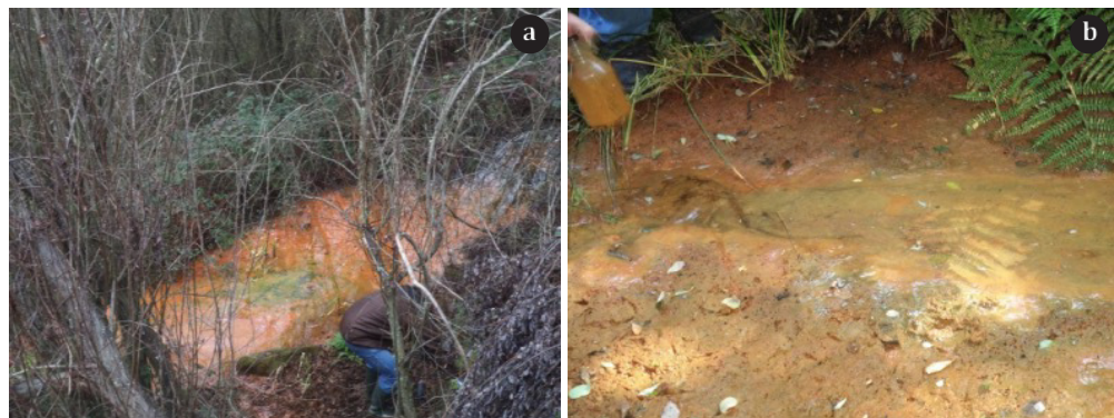
Figure 1 Field images of ochre-precipitates in the mine water receiving creek. a) Pond at the exit of the gallery; b) Boco creek, \approx 500 m downstream the gallery
