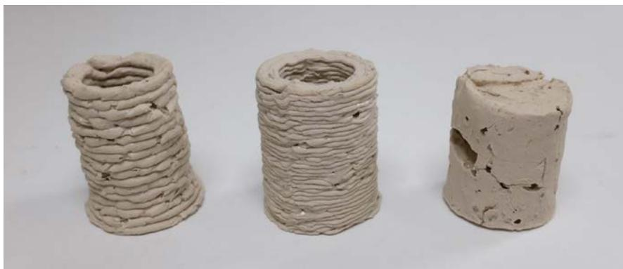
Figure 6: Tests of ceramic paste with fiberglass (5%).
