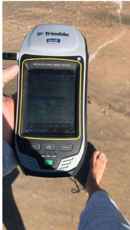
Figura 2-29 Recetor Trimble Geo XR
