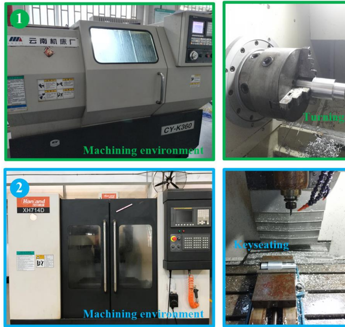
Fig.12 The coupling shaft in machining
