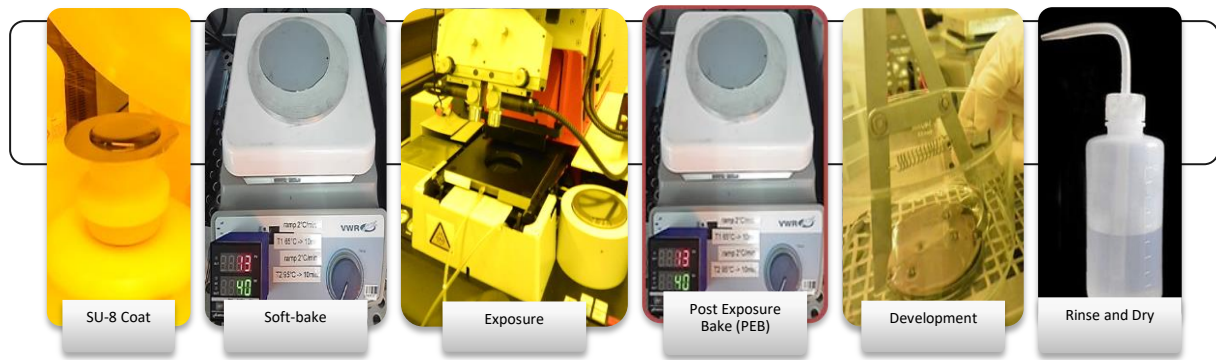
Figure 21: Schematic diagram of the main steps of the photolithography process.
