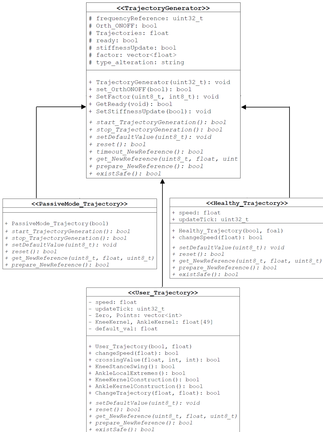
Figure 4.10: Class diagram that displays the classes responsible to generate the reference trajectories.
