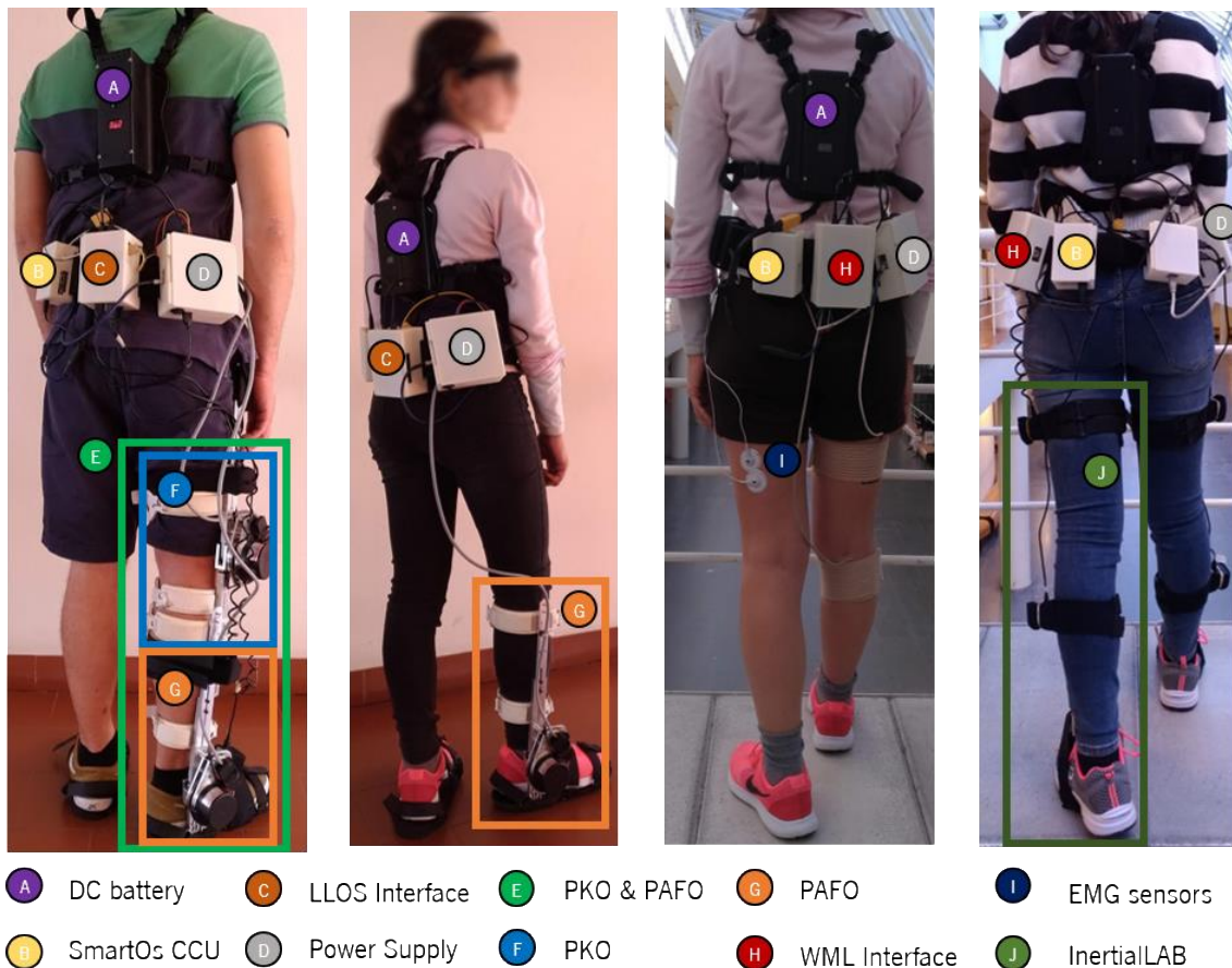
Figure 3.2: SmartOs system overview. Adapted from [61].
