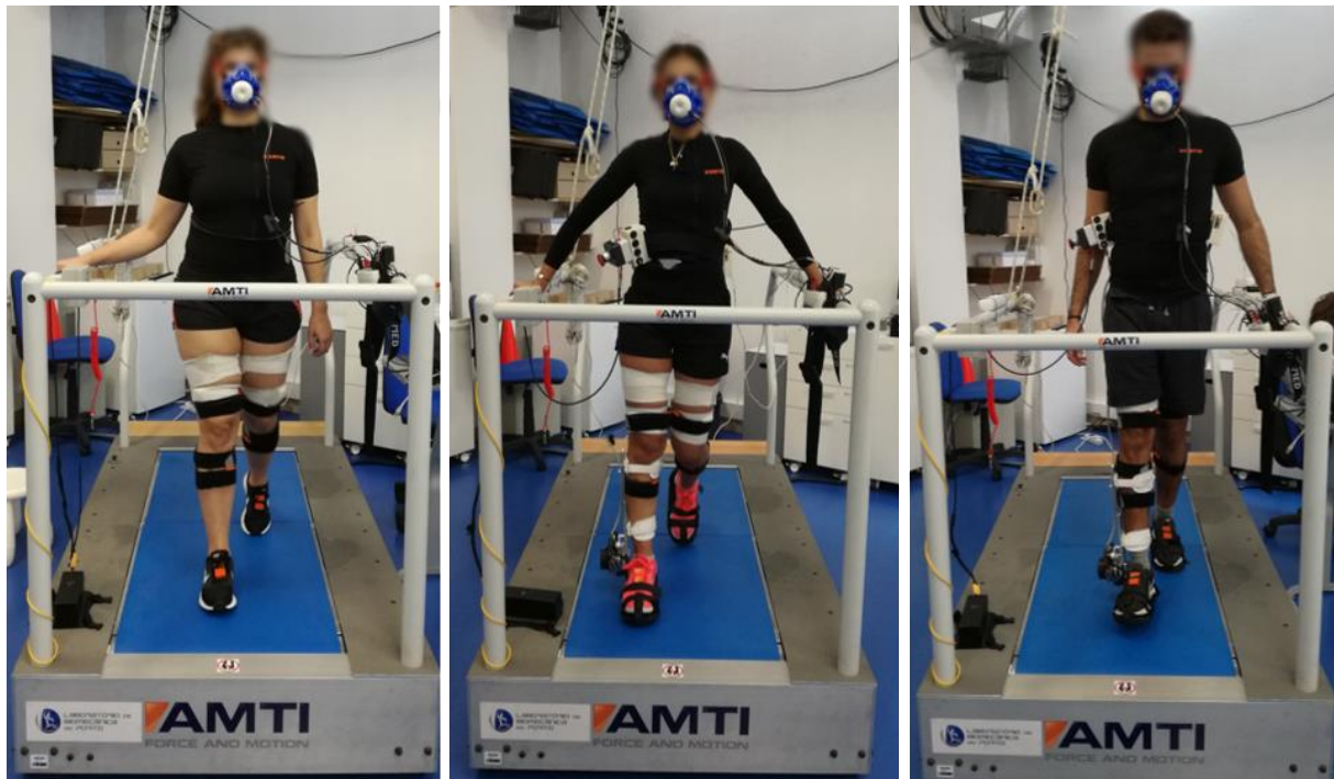
Figure 6.6: Setup for the experimental study to evaluate the energy consumption with and without an orthotic device and for machine learning purposes.
