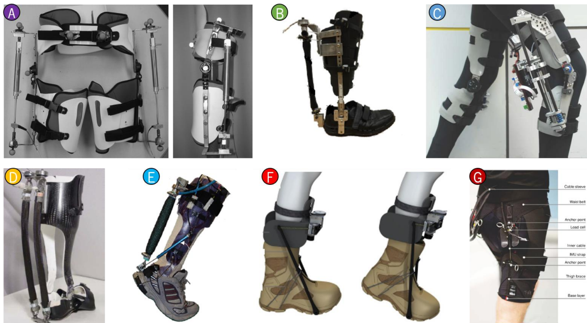
Figure 2.3: Single joints Lower-limbs devices: (A) Pneumatic hip orthosis [23], (B) Pneumatic AFO orthosis [24], (C) MIT PKO orthosis [25], (D) Pneumatic AFO [26], (E) Pneumatic AFO [27], (F) Cable-based ankle-foot exoskeleton [28], and (G) Cable-based hip orthosis [29].
