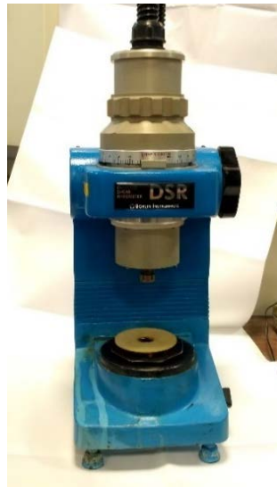
Figure 17 – Dynamic Shear Rheometer (DSR) by Bohlin Instruments
