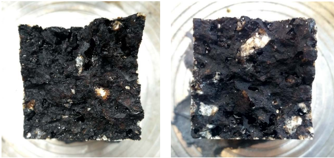
Figure 64 – (a) Specimen failure at +20 °C; (b) Specimen failure at +5 °C
