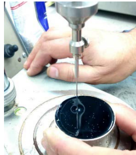
Figure 13 – Bitumen penetration test
