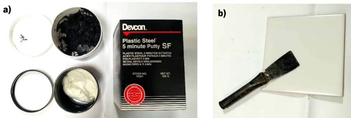
Figure 30 – (a) Bonding agent; (b) Mixing board and spatula
