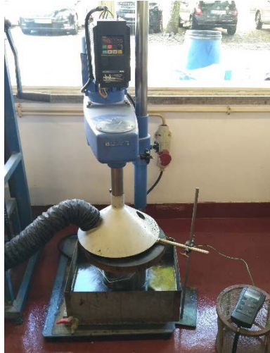
Figure 11 – High shear mixer IKA – T5 Ultra Turrax Basic
