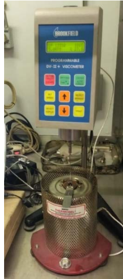
Figure 15 – Brookfield rotational viscometer, model DV-II+Pro
