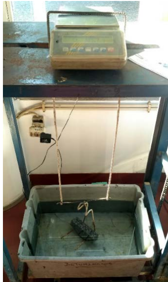
Figure 29 – Bulk density weighing apparatus
