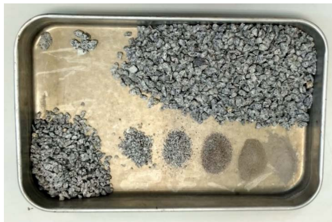
Figure 7 – Grain size distribution for the 4/10 aggregate
