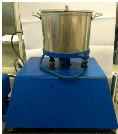
Figure 26 – Pycnometer and vibrating table
