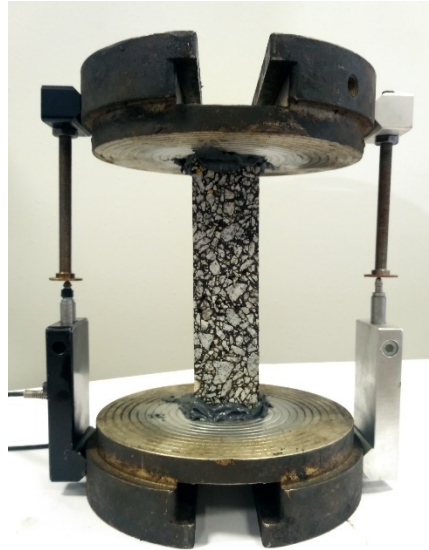
Figure 33 – Specimen glued to connectors and measuring devices (LVDT)
