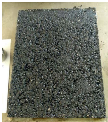
Figure 25 – Asphalt mixture slab after compaction
