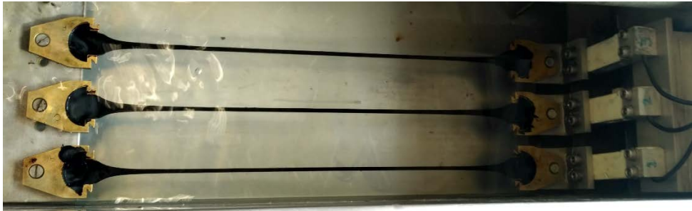
Figure 21 – Elongation of force ductility specimens
