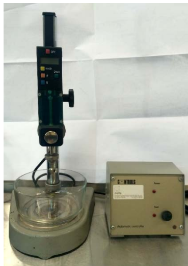
Figure 14 – Semiautomatic penetrometer, Control Groups, model 81-B0101/D
