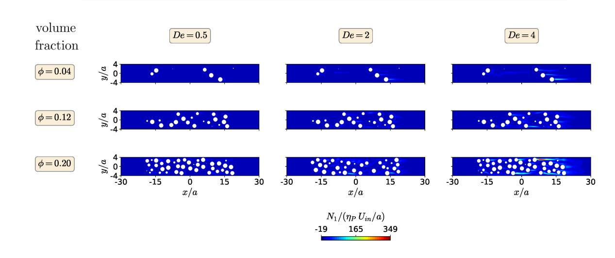
These are DNS of the normal stress difference,  $N_1(\mathbf{x}, De, \phi, Re) =$  $au_{xx}- au_{yy}$  , for random arrays of spheres immersed in a fluid following a quasi-linear viscoelastic Oldroyd-B model. What is the drag law for dense systems? And, for the non-linear viscoelastic Giesekus model?
