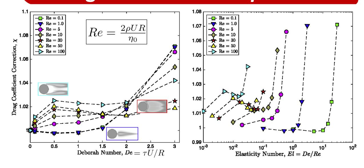
This is for the quasi-linear viscoelastic Oldroyd-B model (with relaxation time au and viscosity  $\eta_0$  ), but what happens for the nonlinear viscoelastic Giesekus model?
