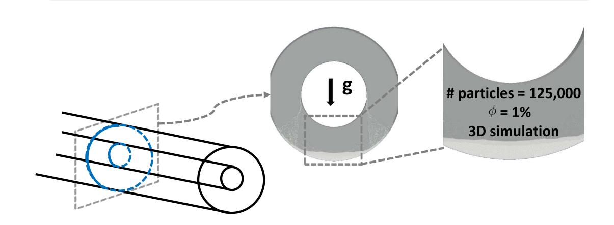
This is particle sedimentation for a Newtonian fluid, but how would it look like for a viscoelastic fluid?
