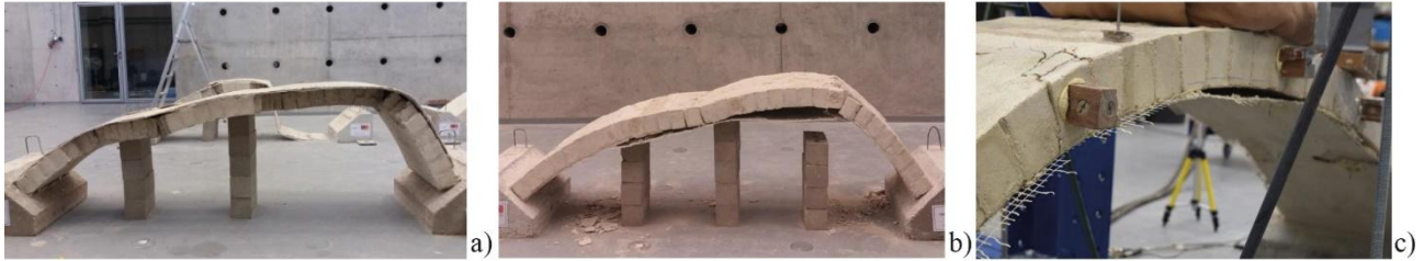
8 9 10 11 12 13 14 15 16 17 Figure 4 Collapse due to the TRM detachment: a) arch strengthened at the extrados (SE1); b) arch 18 strengthened at the intrados (SI1); c) Repaired arch strengthened at the intrados (RSI1). 19
