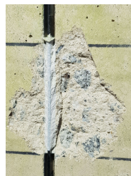
I-FA + C-C + CS Debonding at CFRP- Adhesive interface and cohesive failure of concrete with concrete splitting
