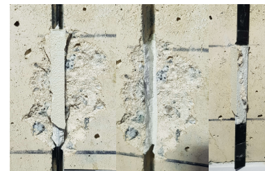
C-A + CS Cohesive failure of adhesive with concrete splitting
