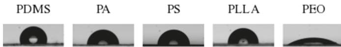
Figure 3. Water droplet over the surfaces of PDMS, PA, PS, poly-L-lactide acid (PLLA) and Polyethylene oxide (PEO) illustrating the hydrophobicity of the materials.
