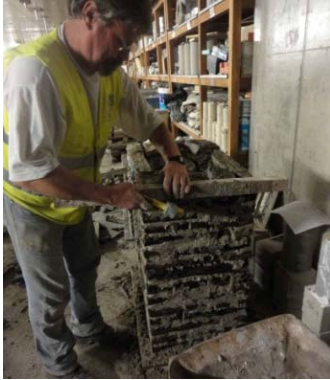
Figure 5 – (a) Construction of the walls (b) Final aspect of the wallet P4
