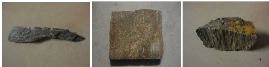
Figure 2 - Appearance of schist stones after cutting with hammer and pointer
