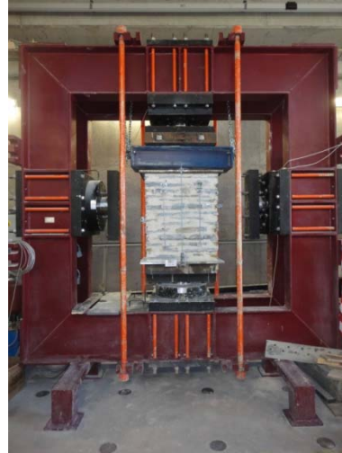
Figure 7 – Test setup of the walls: scheme and testing machine
