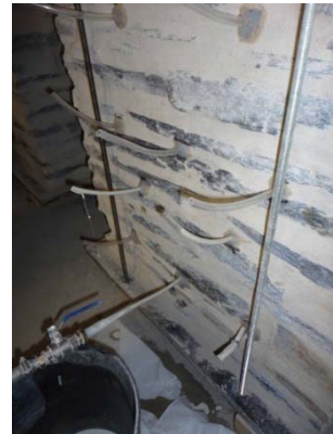
Figure 6 – (a) Wallet final aspect before grouting; (b) Introduction of grout in the pressure pot; (c) Injection of the walls
