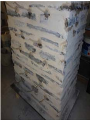
Figure 6 – (a) Wallet final aspect before grouting; (b) Introduction of grout in the pressure pot; (c) Injection of the walls
