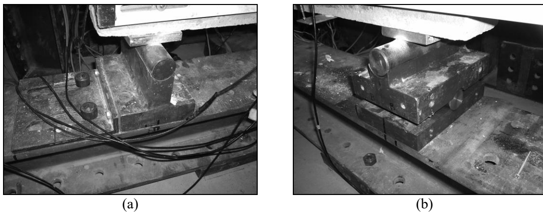
Fig. 2. Details of the boundary conditions of masonry beams: (a) fixed support; (b) free support.
