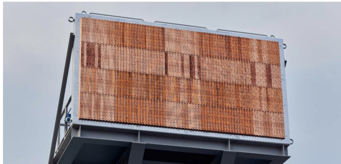
Prototype of resin-injection-molded waveguide array antenna
