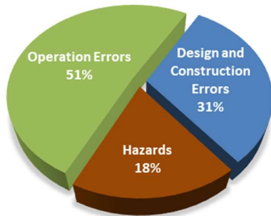
Figure 1. Leading causes of failure for reinforced concrete bridges [2]
