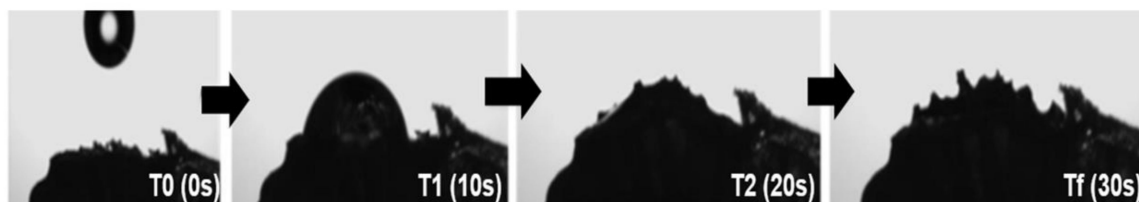
Figure 5. Hydrogel swelling process (images from goniometer assay using Xanthan-Chitosan hydrogels and distilled water). Source: Batista et al. (2019) with permission [18].
