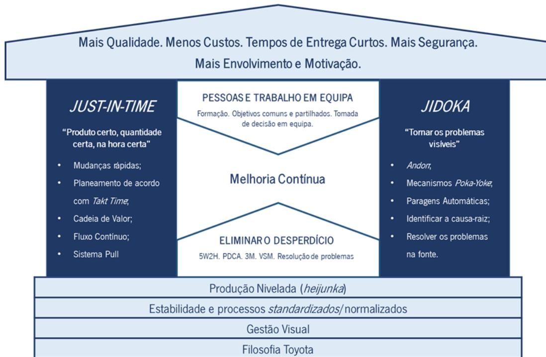
Figura 5: Casa do Toyota Production System (adaptado de Liker (2004))
