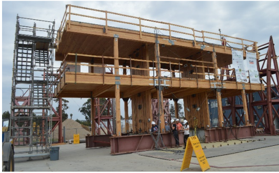
Figure 1: Overview of shake-table specimen tested in 2017. The middle floor level consists of a CLT diaphragm. The roof level consists of a CLT-concrete composite diaphragm.
