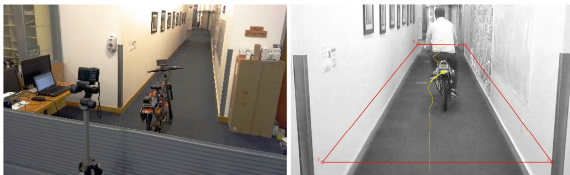
Fig. 13. Left: experimental setup temporarily established during night time, in one of the corridors of MIT Computer Science and Artificial Intelligence Laboratory. Right: tracking the bicycle on the video, as a reference for data consistency check.
