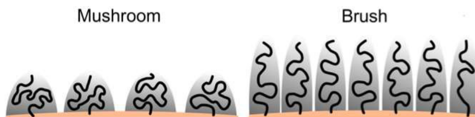
Figure 2 | Schematic representation of nanoparticle surface functionalized with PEG chains in mushroom and brush conformations [From Loureiro et al. , 2016 [2]].
