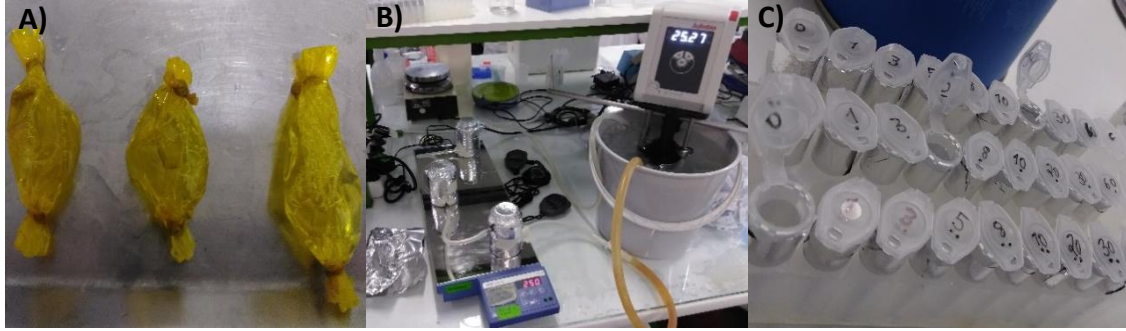
Figure 4. Representative image of A) dialysis membranes, B) experimental mechanism, and C) collection of samples used in release kinetics assays
